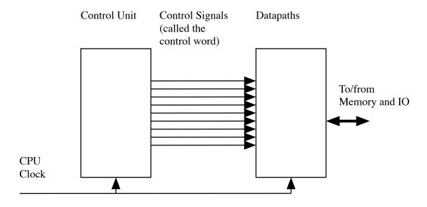
(We continue to assume a single core. A multi-core CPU actually has two or more instances of the Control Unit an Data Paths)
